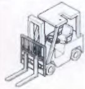
**Class 2 -Electric Motor Narrow Aisle. Code 1**
